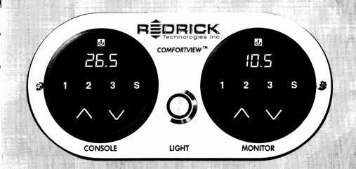
**\*NOTE:** Holding the "S" button for too long after the height displays are unlocked can result in the touch controls returning to locking mode.
